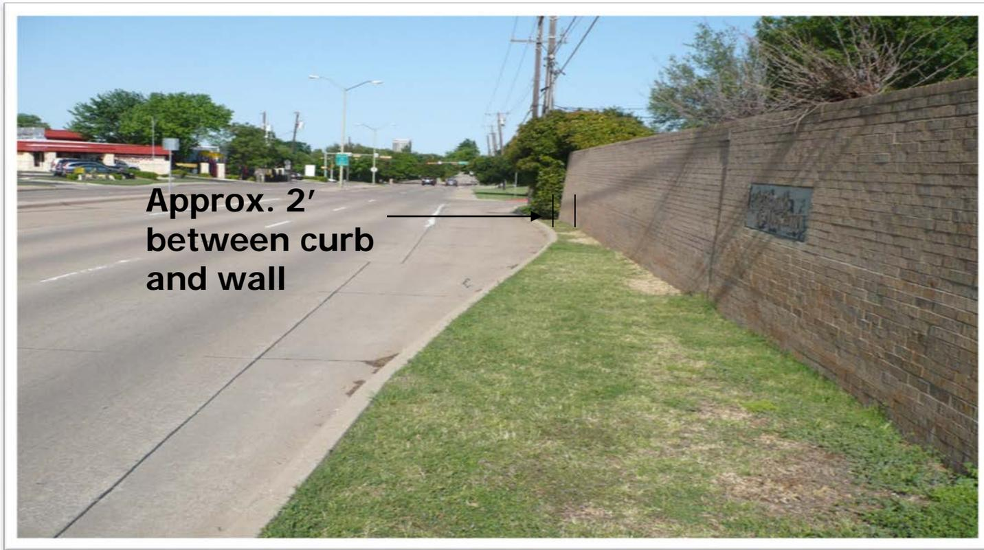
Lack of right-of-way and obstructing screening wall
