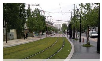
These light rail tracks run above grass, increasing pervious surface while also improving overall aesthetics
