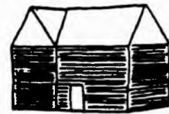
WOODEN WALL CLADDING
