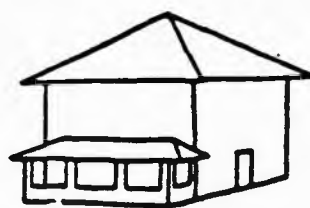
HIPPED ROOF, SYMMETRICAL, NO FRONT ENTRY
