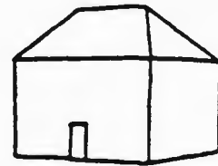
HIPPED ROOF WITHOUT FULL-WIDTH PORCH
