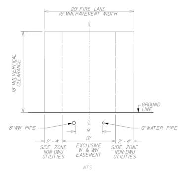
Figure 6.2.1 Shared Access Easement Section-Cut
