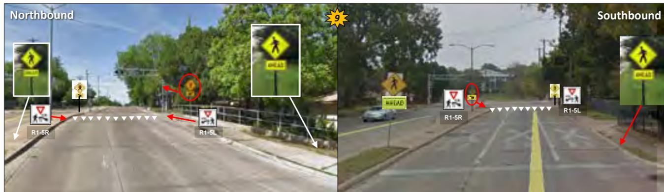
Move the existing pedestrian crossing sign to the north, closer to the crosswalk. Install a pedestrian crossing sign in the median. Install pedestrian advance crossing warning signs ahead of the existing pedestrian crossing sign.
