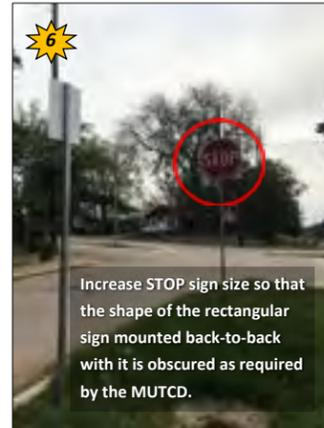
Increase STOP sign size so that the shape of the rectangular sign mounted back-to-back with it is obscured as required by the MUTCD.
