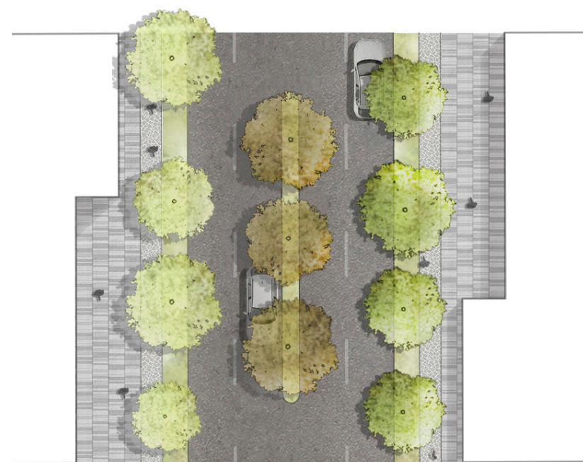
TYPICAL 2-WAY ROAD TWO 11'-0" CAR LANES EACH DIRECTION 4'-0" LANDSCAPED MEDIAN 8' LANDSCAPE EDGE AT STREET 5' SIDEWALK OUTDOOR RETAIL SEATING
