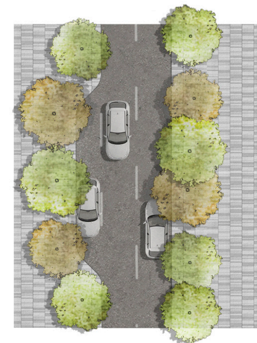
ONE LANE ROAD ONE 11'-0" CAR LANE EACH DIRECTION 8'-0" PARKING LANE ONE SIDE AS NEEDED NO MEDIAN LANDSCAPE AT PAVEMENT EDGE OPEN PAVED AREAS
