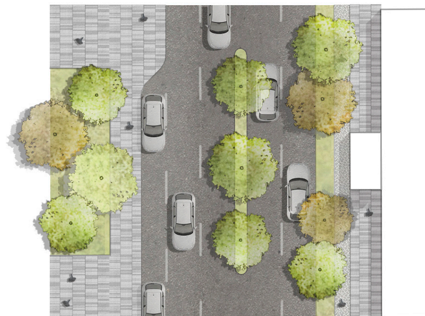
2-WAY ROAD WITH 1-SIDED PARKING TWO 11'-0" CAR LANES EACH DIRECTION 8'-0" PARKING LANE 4'-0" LANDSCAPED MEDIAN 8' LANDSCAPE EDGE AT STREET 5' SIDEWALK
