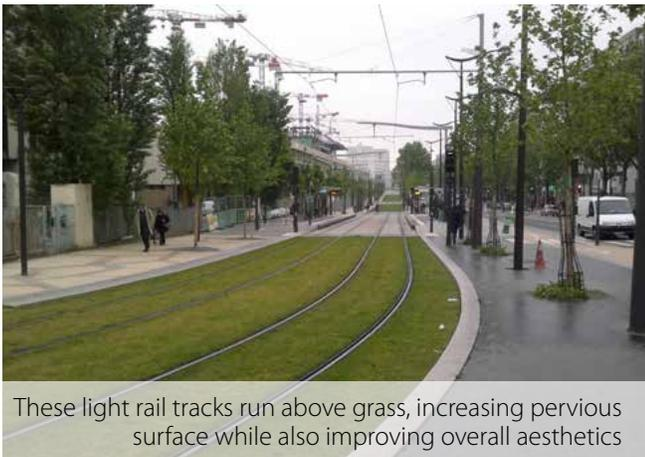
These light rail tracks run above grass, increasing pervious surface while also improving overall aesthetics
